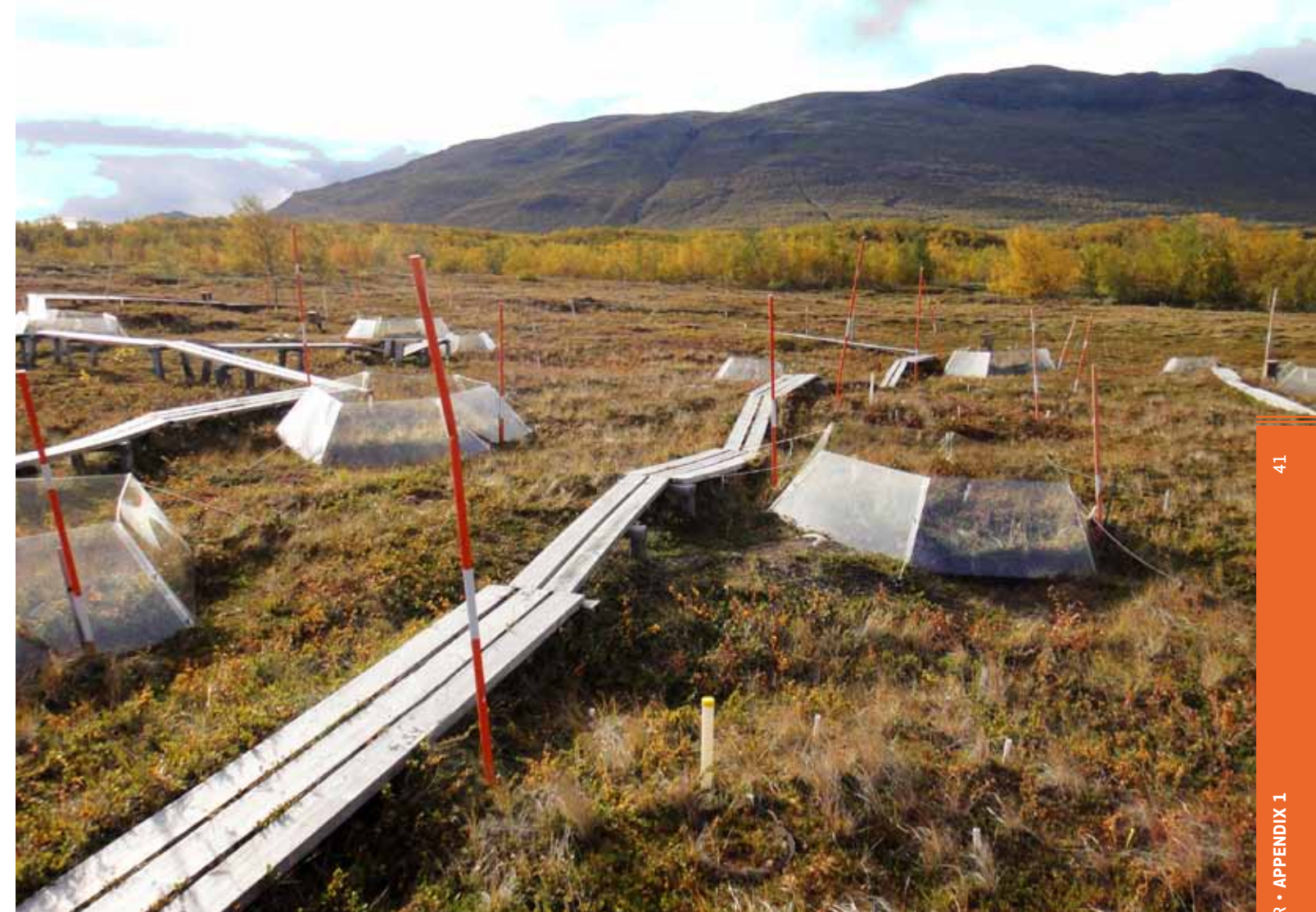
Open-topped perspex chambers are widely used in ecology to simulate effects of climate warming. Here from a workshop in Abisko, Swedish Lapland. Photo: Hilary Birks.
